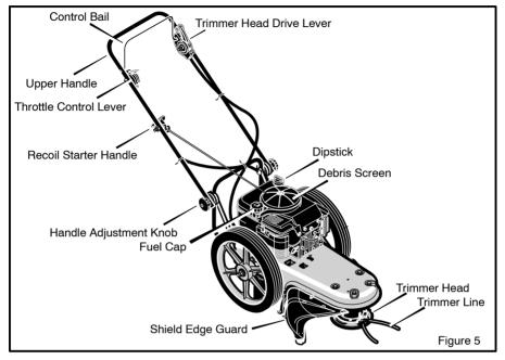
**Trimmer Head Drive Lever** – Engages the rotation of the trimmer head.
